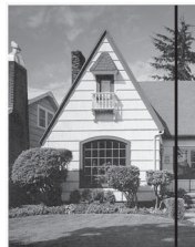
When there is a spot of dirt or correction fluid on the glass strip the scanned sample shows a vertical line.
